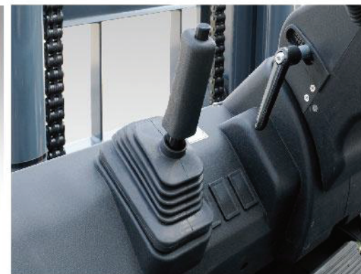
Ratchet type parking brake
